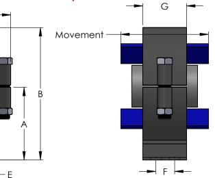
Spider Spacers Center Pipe In Housing And Are Sized To Allow Insulation To Be Packed Around Pipe
