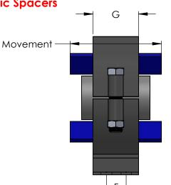
Spider Spacers Center Pipe In Housing And Are Sized To Allow Insulation To Be Packed Around Pipe
