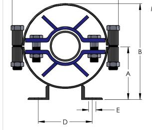
Provides Lateral Stability To The Pipe To Prevent "Bowing". Guides Are Not Designed To Support The Weight Of The Pipe.
