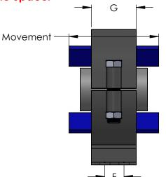
Spider Spacers Center Pipe In Housing And Are Sized To Allow Insulation To Be Packed Around Pipe
