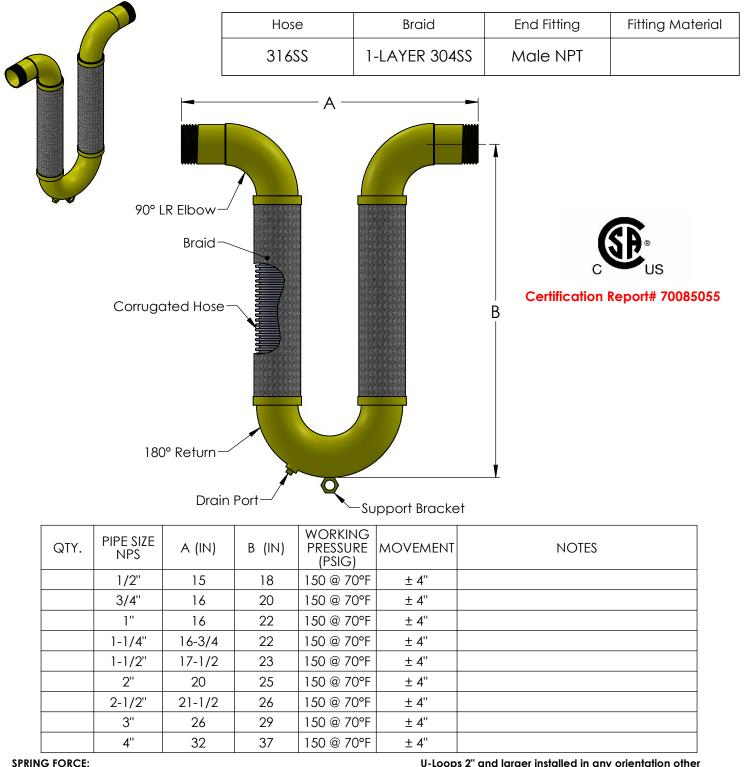
\*These values reflect the total force required to move the U-Loop its full rated movement for 150 PSI @ 70°F. All dimensions are in inches.
