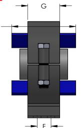
Spider Spacers Center Pipe In Housing And Are Sized To Allow Insulation To Be Packed Around Pipe
