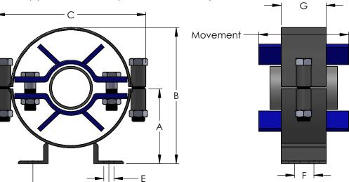
Spider Spacers Center Pipe In Housing And Are Sized To Allow Insulation To Be Packed Around Pipe
